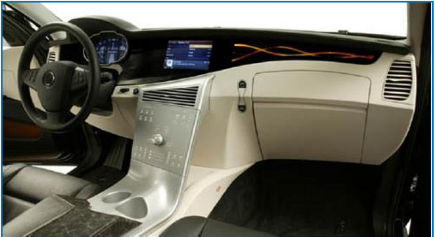
These panels are produced using the InMold Decoration technique (IMD) in which images are printed on flat sheets of plastic film before being thermoformed into a 3D shape and inserted in the cavity of an injection mold tool where they become fully decorated rigid panels. This technique was developed for the automotive industry in the 1990s and was then adopted by the consumer electronics market and the cellphone market in particular.
