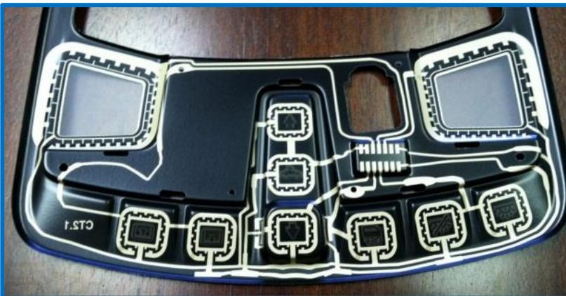
Printing of these sensor elements requires conductive inks which can be successfully thermoformed into 3D shapes without losing any significant conductivity and a comprehensive understanding of how the sensor shape will distort as it changes from 2D to 3D.
